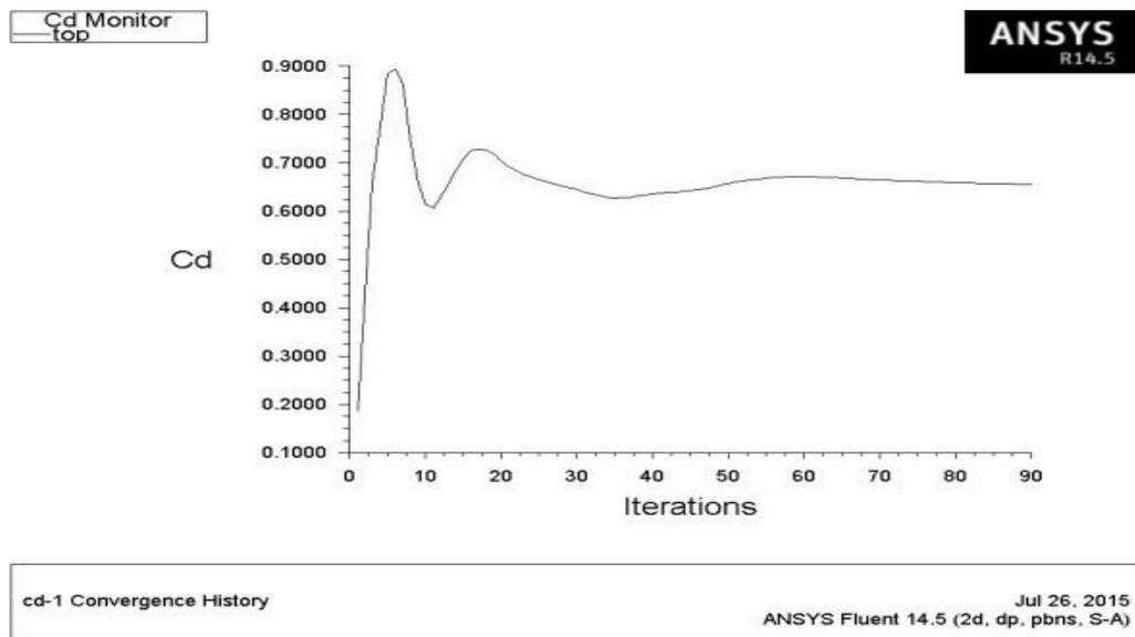
Fig 5.7 Coefficient of Drag curve of NACA 2412 airfoil
