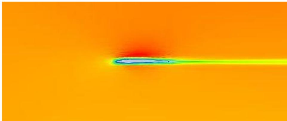
Fig 5.5: Velocity contours of NACA 2412 airfoil
