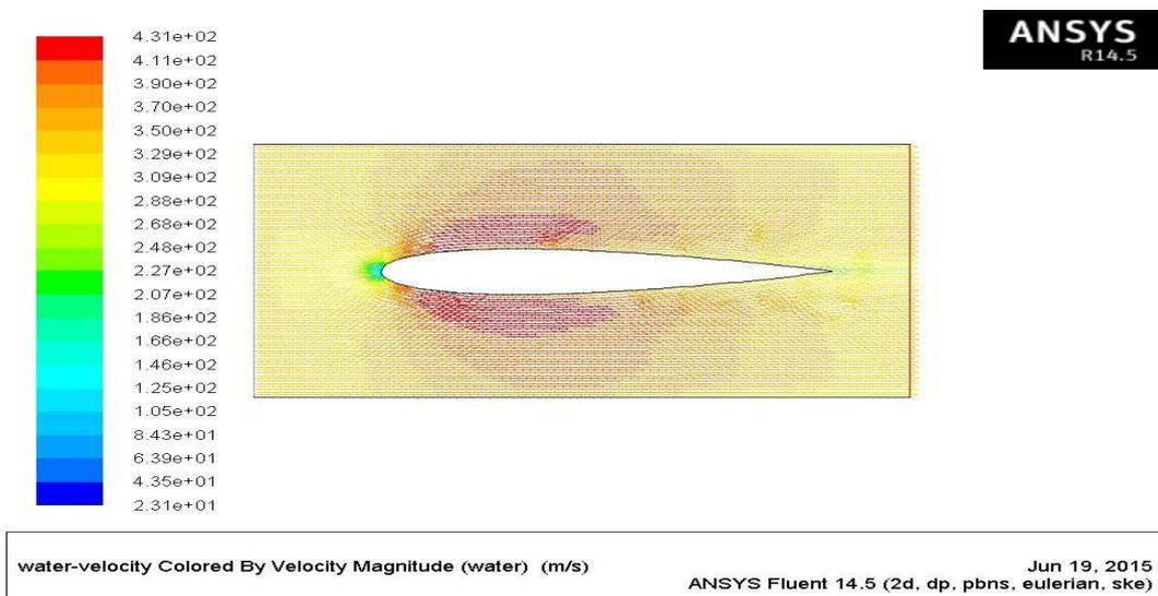
Fig 5.1: Velocity contours of NACA 0015 airfoil in CFD
