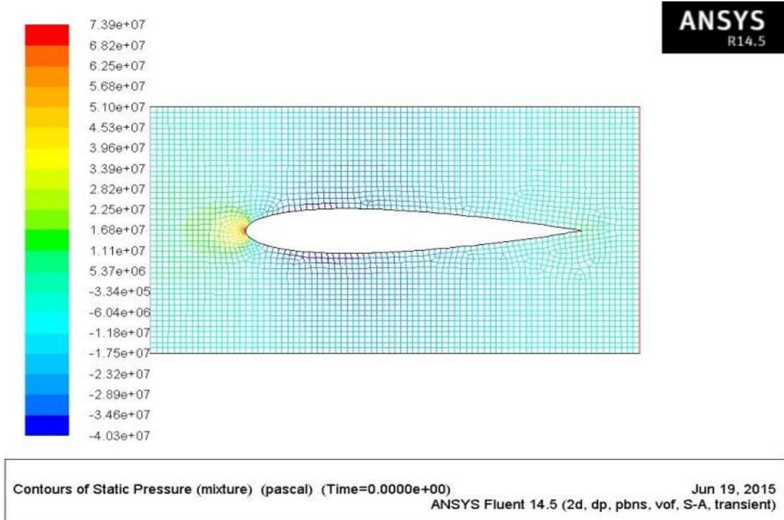
Fig 5.2: Pressure contours of NACA0015 airfoil in CFD
