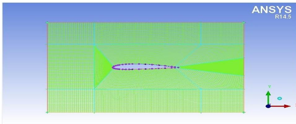
Fig 4.2: Mesh generated airfoil in ICEM CFD
